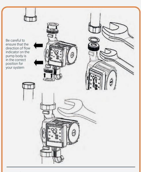
**Attention:** Fit the two seals between the pump and the pump valves.
