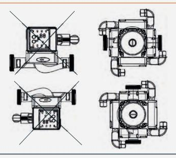
**Attention:** The pump MUST be installed with the motor shaft in the horizontal position to prevent air from collecting within the pump head.
